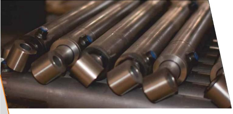
Imported rods with chrome coating are used in hydraulic cylinders (with 25 microns thickness) preventing from rust, staining, dyeing on the surface, and wear of sleeves with honed surface; sealing joints and scrapers are provided with improved profile, which ensure a long operating period for the cylinders.
