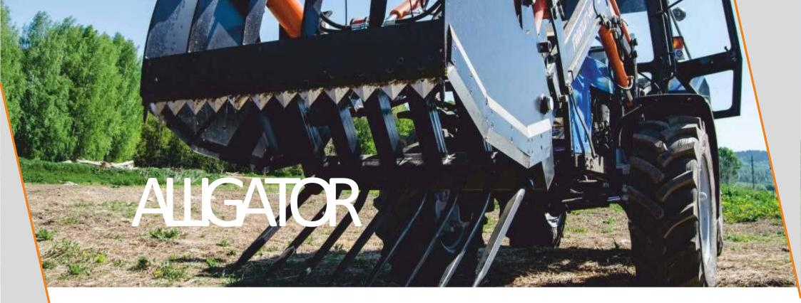
Alligator silage cutter is designed for silage batch extraction. Top and side cutting blades ensure clean cut, preventing air ingress into the silage. Closed type design prevents spilling and loss of silage mass.
