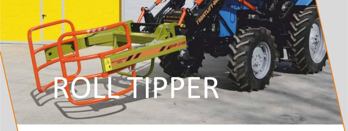
Roll tipper is designed for rolls gripping, handling and storing; ensures thier lifting and lowering to the height of 3.4 meters (along the bottom edge of the roll) tipping by 90° without damaging package film.
