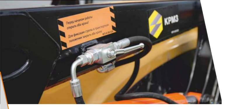
Cranes with hydraulic lock ensure security in tractor driving on public roads in accordance with the Russian regulations.
