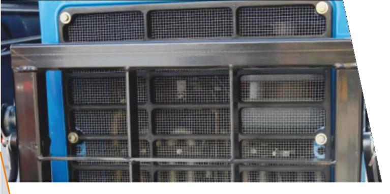
Protective radiator guard reliably protects the front part of the tractor from damage.
