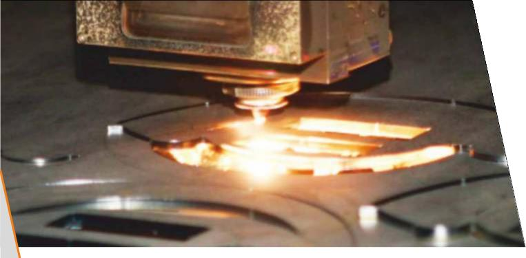
It is produced on Italian production line consisting of the machines for laser cutting, precision bending and robot welding and ensures high precision of cutting, 100% assemblability and welds reliability.
